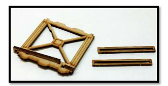
2. Start with a bulkhead, and the two "J" shaped clips. Fit them into the notch near the top (the bulkhead in the pic is upside down for easier visibility) then into the hole, as shown in the picture. They snap fit, and you can add glue if you wish, but it's not needed.
