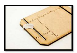
4. Before you slide the bulkheads onto the floors, rub some candle wax on the channels. You can put it on both the floors and the bulkheads. **Skipping this step can lead to broken pieces, frustration, then sadness.** The fits are tight at first, but loosen up a bit over time.
